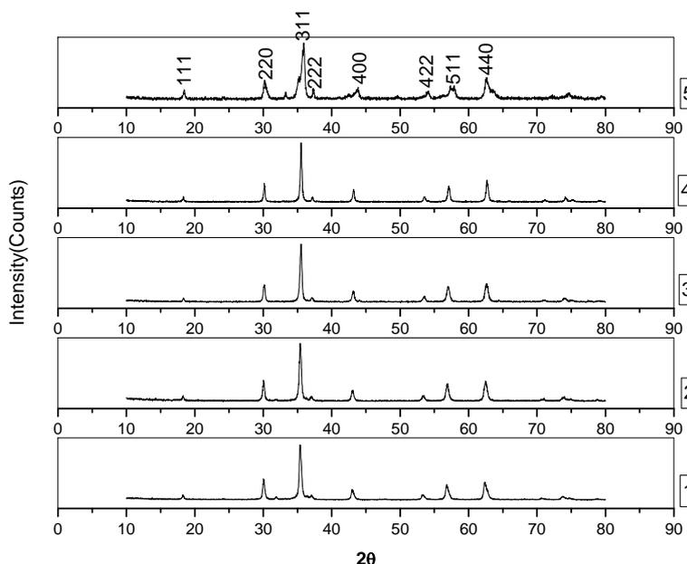
**Fig(1).XRD Pattern of Cu Substituted Ni-Zn Nano-Ferrites**
