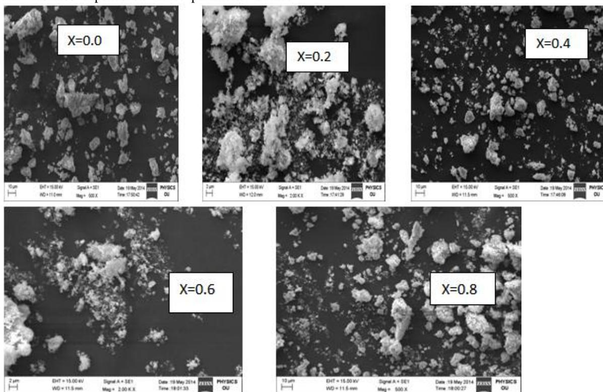
**Fig(2).SEM Micrographs of Ni-Cu-Zn Nano ferrites**
