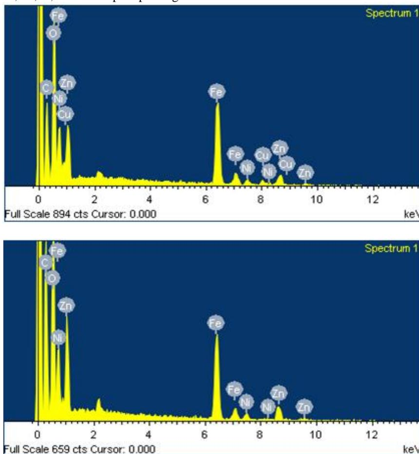
Fig (3).EDS Spectra of Ni-Cu-Zn Nano ferrites
